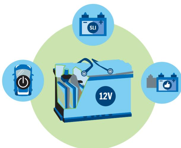
In addition to the battery used for the propulsion of an electric vehicle (usually a lithium-ion one), all plug-in hybrid electric and full electric vehicles require a separate lead battery for functional safety, controls, comfort features and redundancy.
